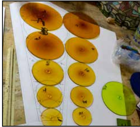
Left: The detail of a quarter section as part of a mockup provided for approval prior to fabricating the stained glass pieces. Center: Steve Brooks produced 300 rondels with variations from light to dark that were used for the inner circle.. Right: The panels laid into the framework. PHOTOS COURTESY B.A. HUDGINS PHOTOGRAPHY
