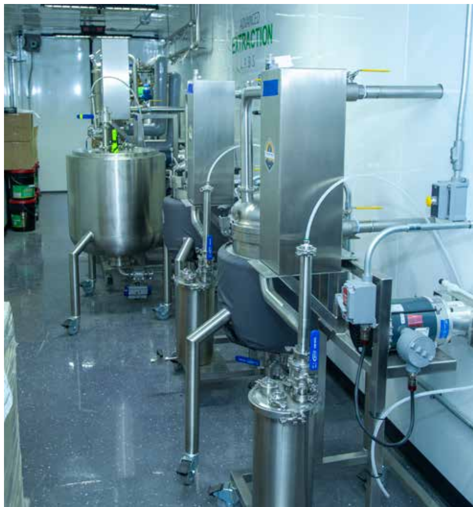
The extraction room at CoPack Industries is where ethanol will be used as a solvent to remove THC and other cannabinoid compounds from cannabis grown at the Springfield business that has been milled, or ground up, in preparation for extraction. The ethanol later will be removed in the distillation process and the resulting THC distillate will be used for on-site infusion of beverages. PHOTO BY STEVE HINRICH.
